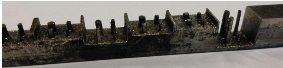
Fig. 4 – Columns generated by using plate type tool for electrical discharge machining.
