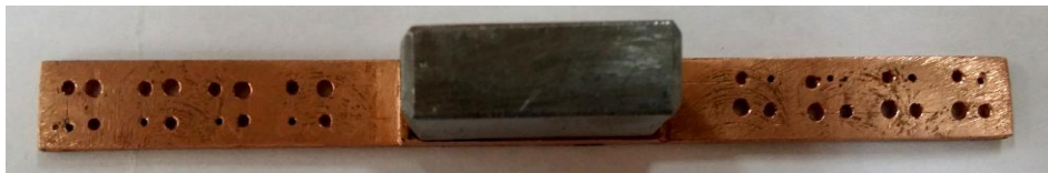
Fig. 3 – Plate type tool electrode used for experimental investigation of the influence exerted by some process input factors on the machining speed at electrical discharge machining of external cylindrical surfaces.
